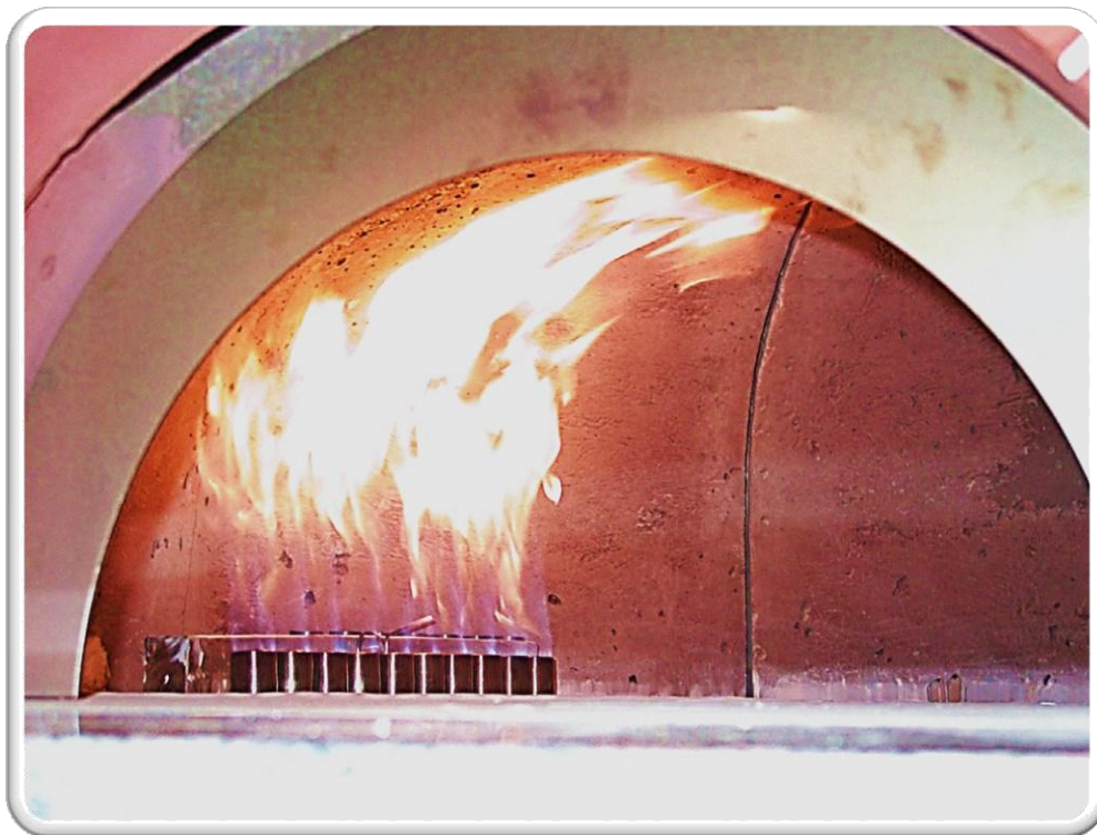
Image of the flame on maximum with power 70% and temperature 420°C
