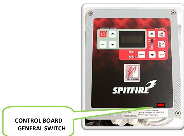
Figure B: burner's controls overview
