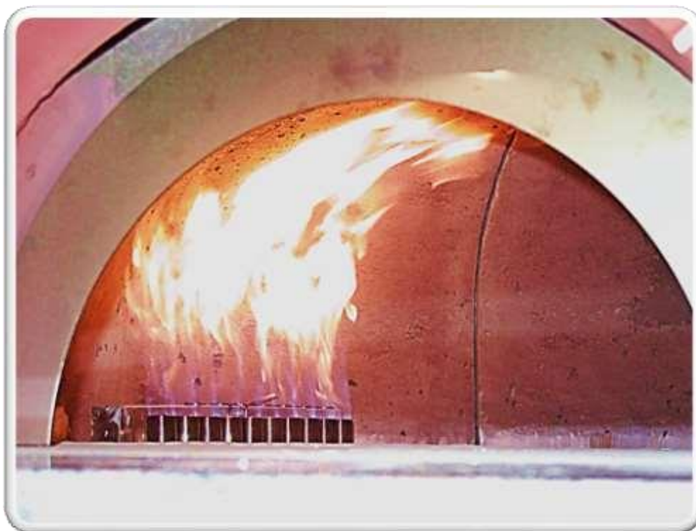
Image with flame at the maximum with power 70% and temperature 420°C
